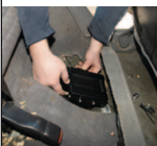
We decided to mount the IC-208H head unit under the rear seat of our '97 Jeep Cherokee, where the factory CD changer would be installed. The carpet already had a cutout, making it easy to remove, and there was a factory heat shield in place to lessen heat transfer from the floorpan.
