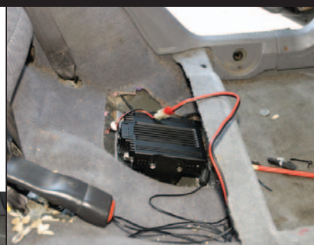
The faceplate separation cable and power supply cables were attached to the radio and routed under the carpet forward to the center console and on to behind the dash.
