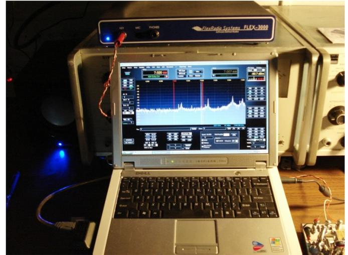
The FLEX-3000 is operated from the computer screen. The unit has no knobs or dials (that's it on top of photo). Note the signals appear continuously as a spectrum scan and all receiver functions are controlled with the mouse. There are controls that no analog equipment has.
